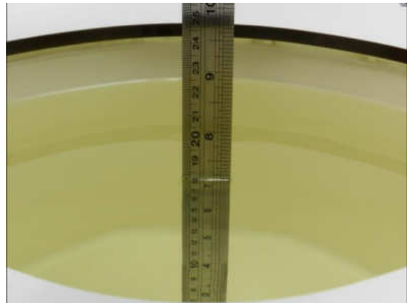
Fig 10.2 Photo of Liquid Height for Body SAR
