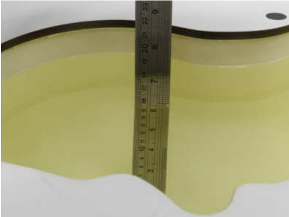
Fig 10.1 Photo of Liquid Height for Head SAR
