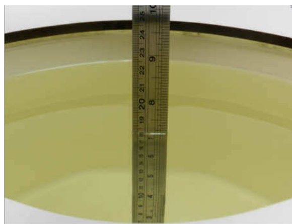
Fig 11.2 Photo of Liquid Height for Body SAR
