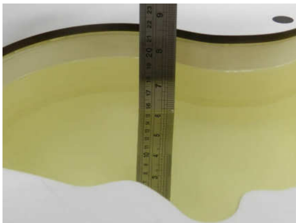
Fig 11.1 Photo of Liquid Height for Head SAR
