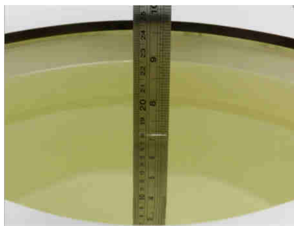
Fig 10.2 Photo of Liquid Height for Body SAR
