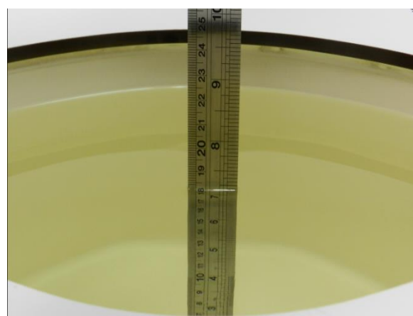
Fig 10.2 Photo of Liquid Height for Body SAR
