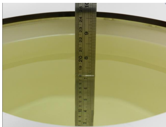
Fig 10.2 Photo of Liquid Height for Body SAR
