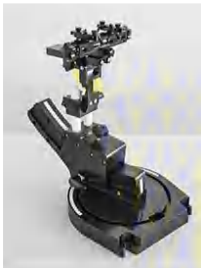
Mounting Device for Hand-Held Transmitters
