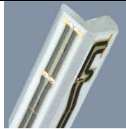
Fig 5.2 Photo of E-field Probe
