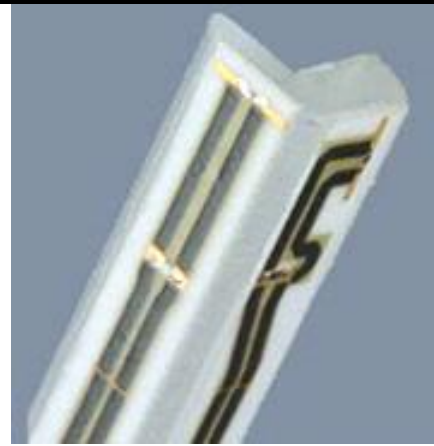
Fig 5.2 Photo of E-field Probe
