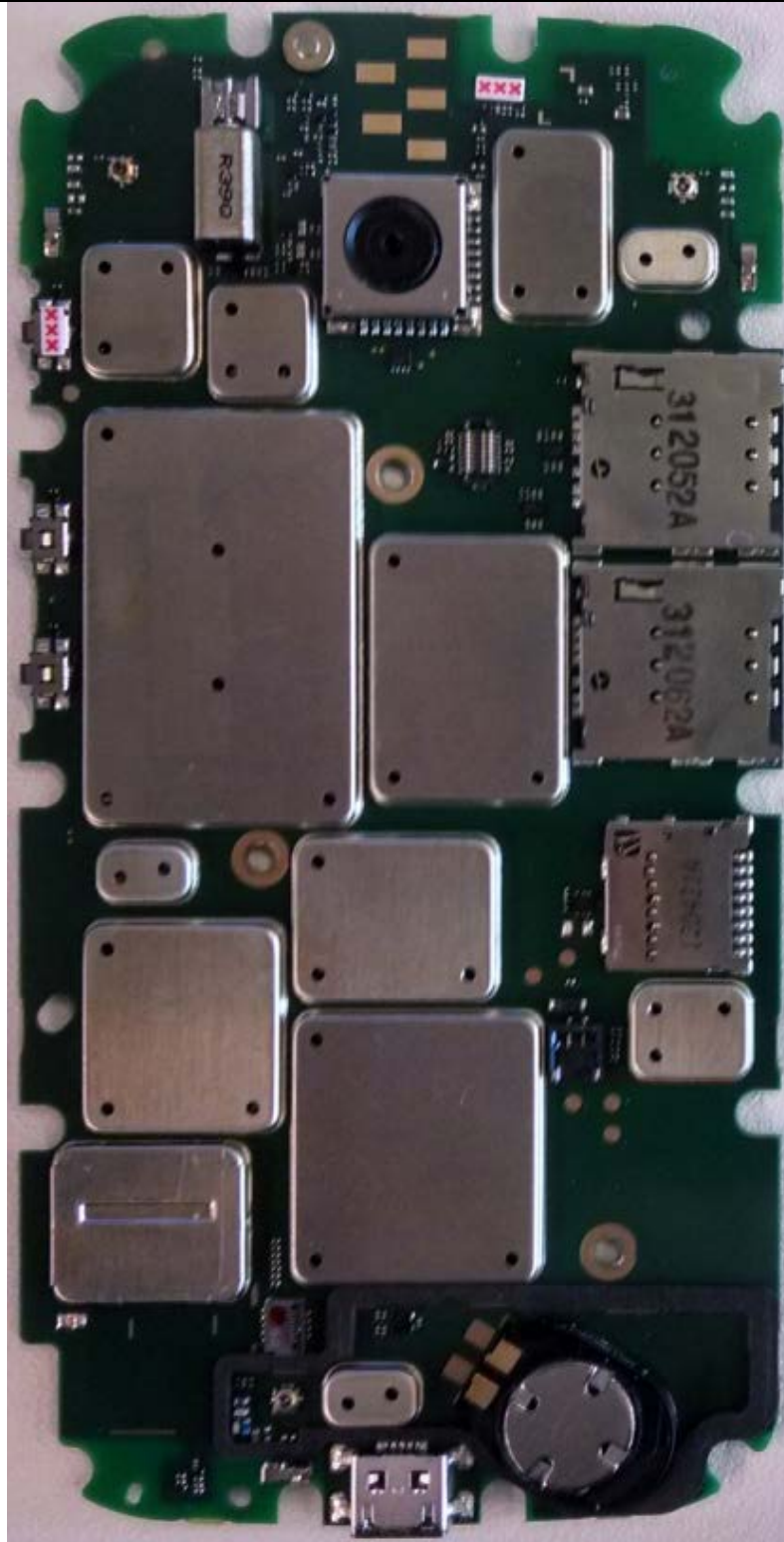
Photograph 9-1: Component Side view of the device's PC Board, Shields in place.
