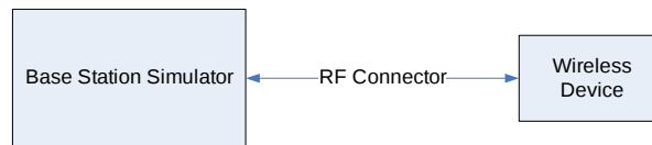
Figure 8-2 Power Measurement Setup
