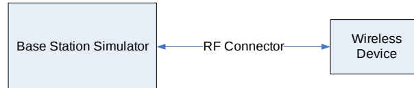
Figure 8-1 Power Measurement Setup
