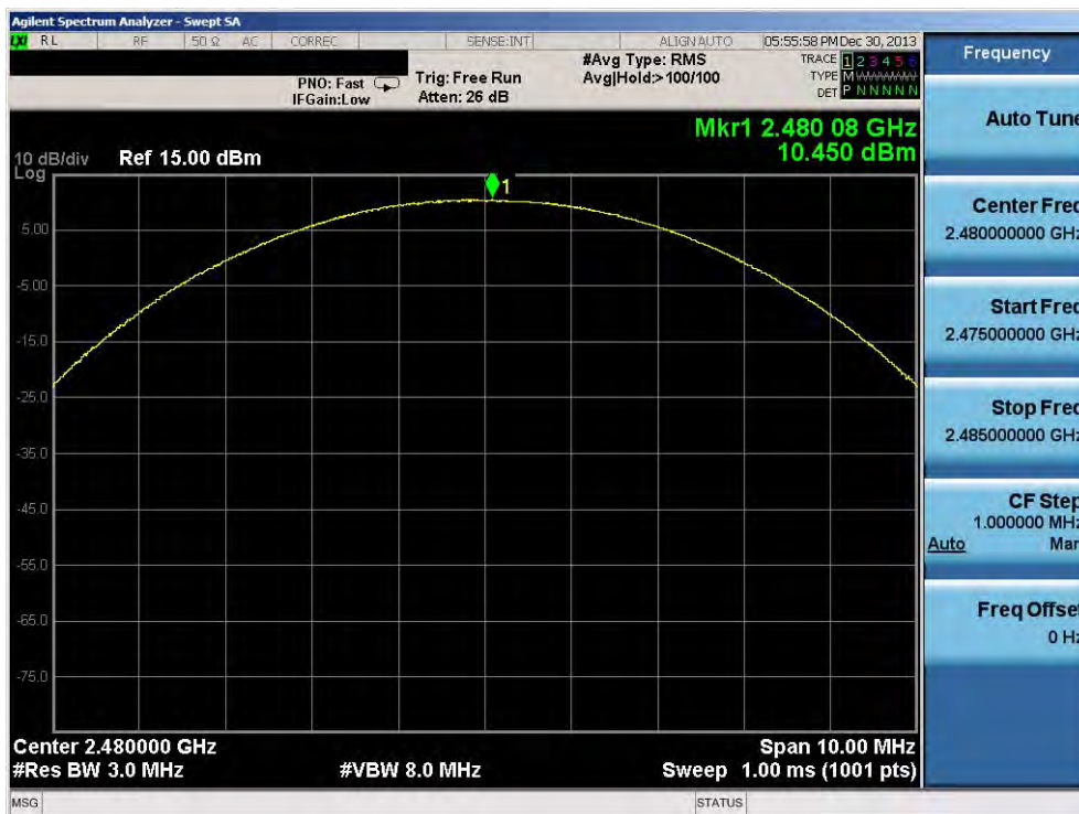
Plot 6-15. Peak Conducted Power (2Mbps – Ch. 78)
