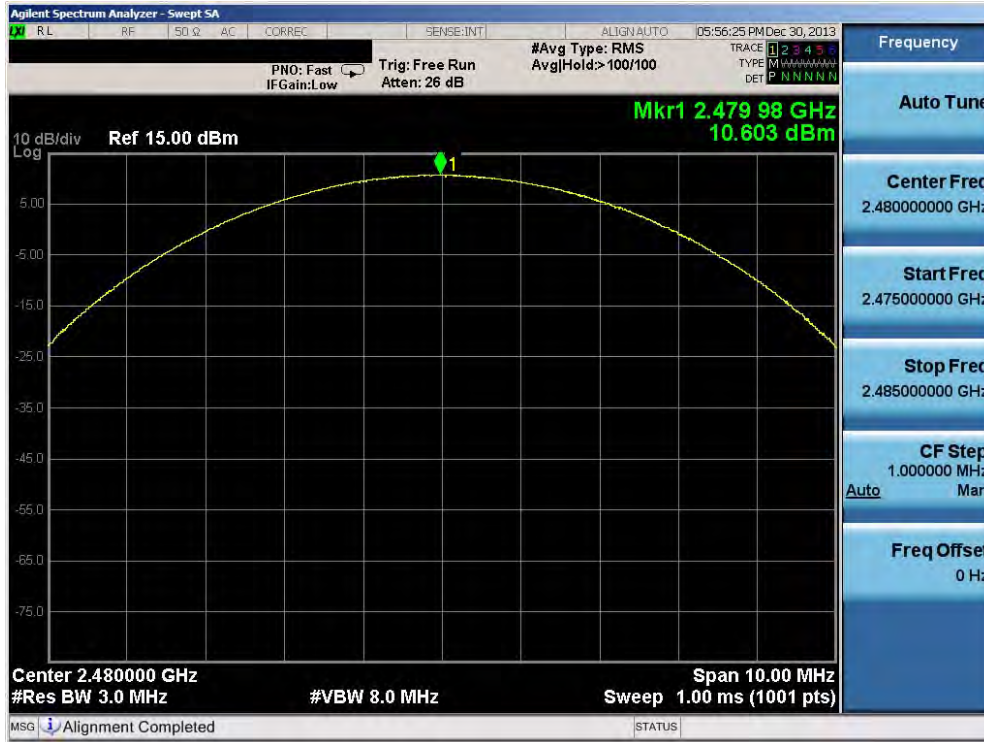
Plot 6-18. Peak Conducted Power (3Mbps – Ch. 78)
