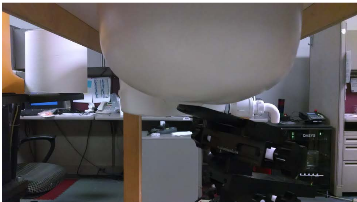
Figure 6: Tilt Position, Top of Head of Phantom
