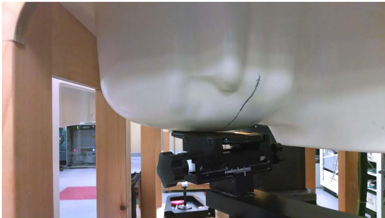
Figure 3: Cheek Position, Front of Head of Phantom
