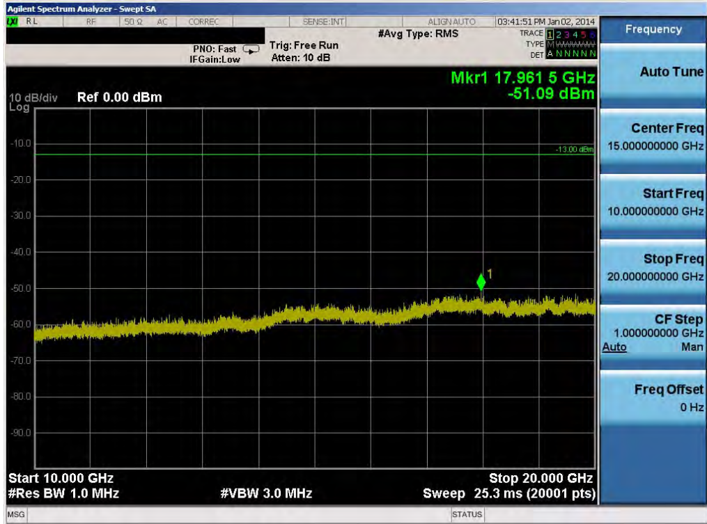
Plot 9-80. Conducted Spurious Plot (20.0MHz QPSK – RB Size 1, RB Offset 0 – High Channel)
