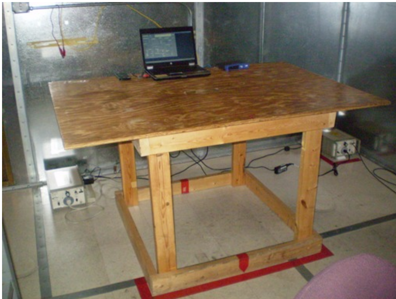
Figure 7B3-1: Test Configuration – AC Line (Part 15 Computing Device).
