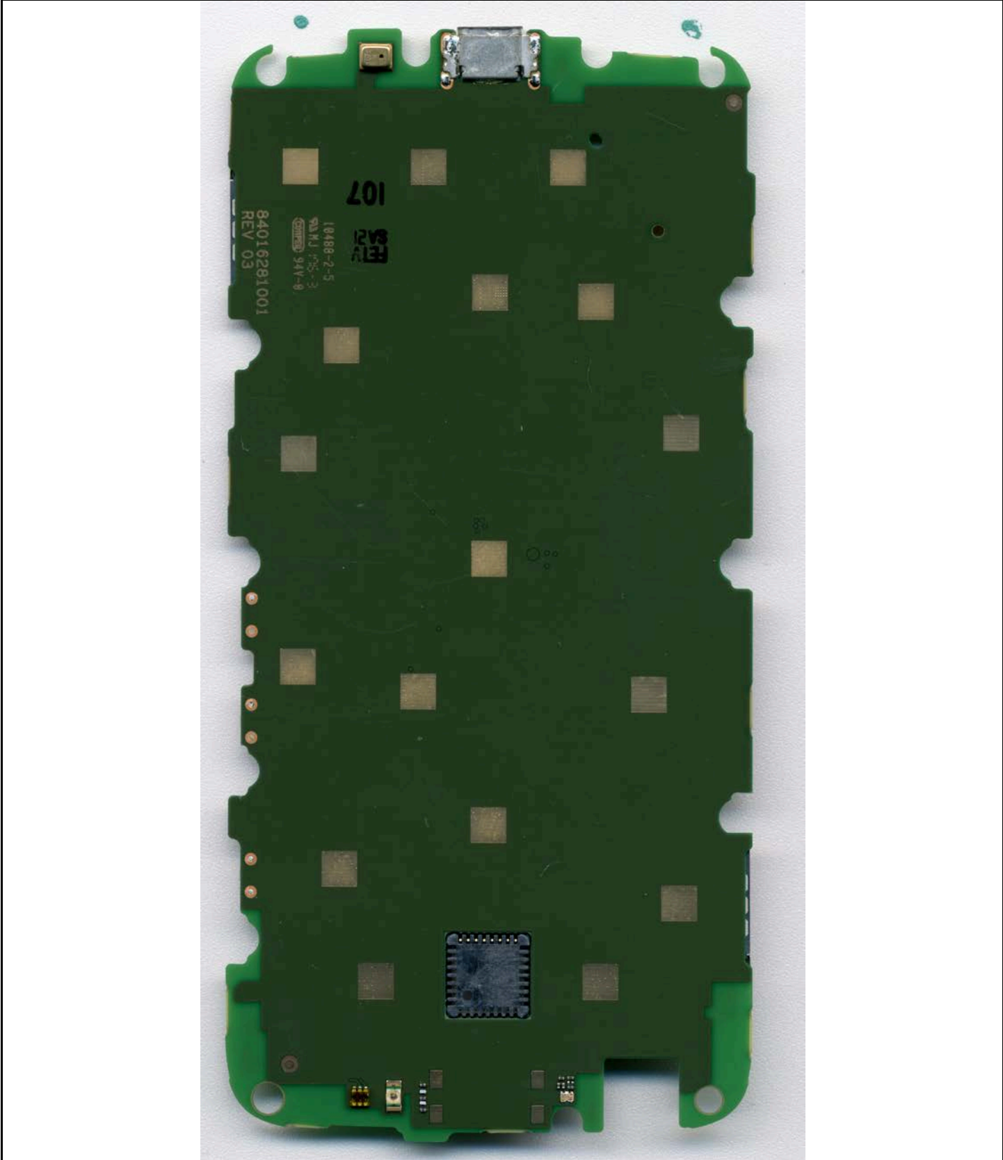
Photograph 9-2: Keypad side view of the device's PC Board.
