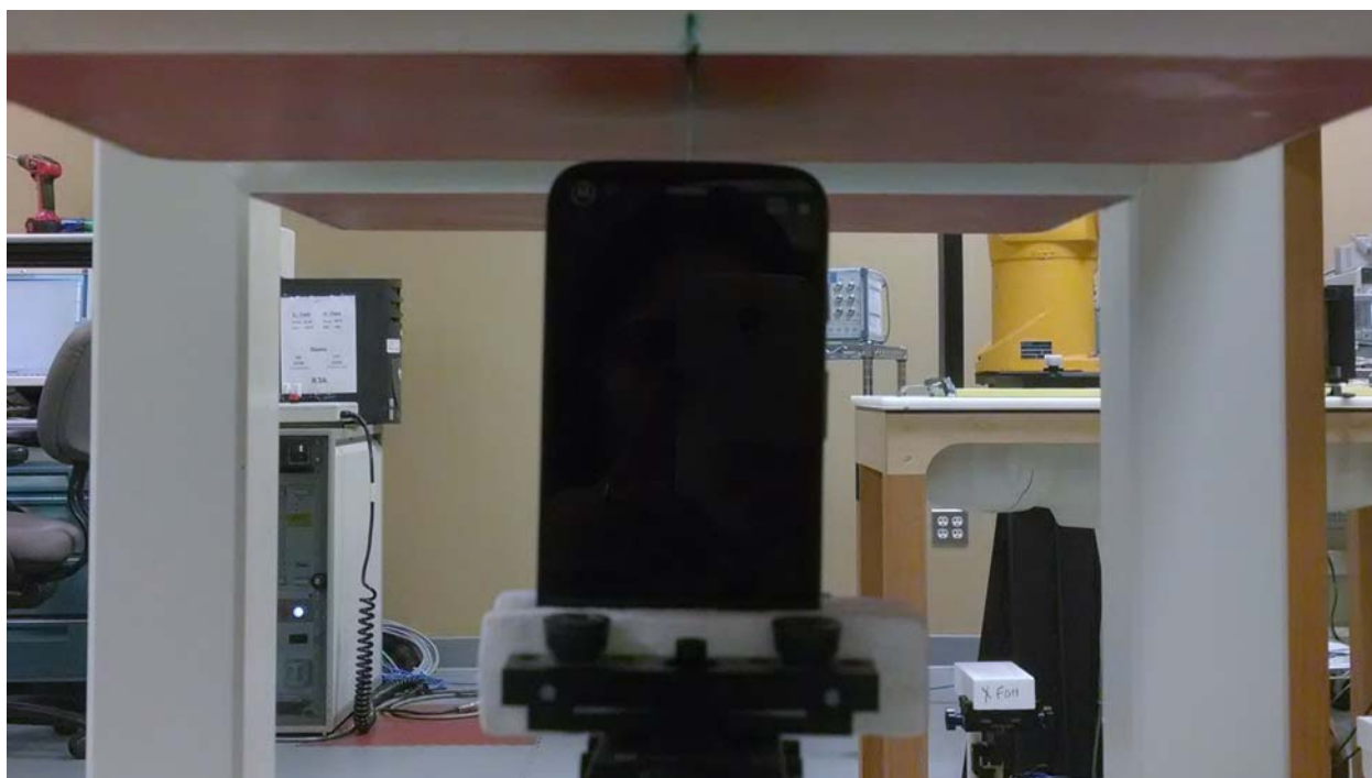
Figure 9: Mobile Hotspot Position, Short Edge of Phone facing Phantom (10 mm separation)
