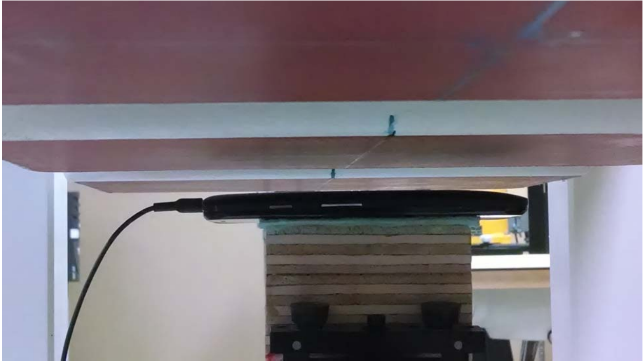
Figure 7: Body Position (15 mm separation, with audio cable shown)
