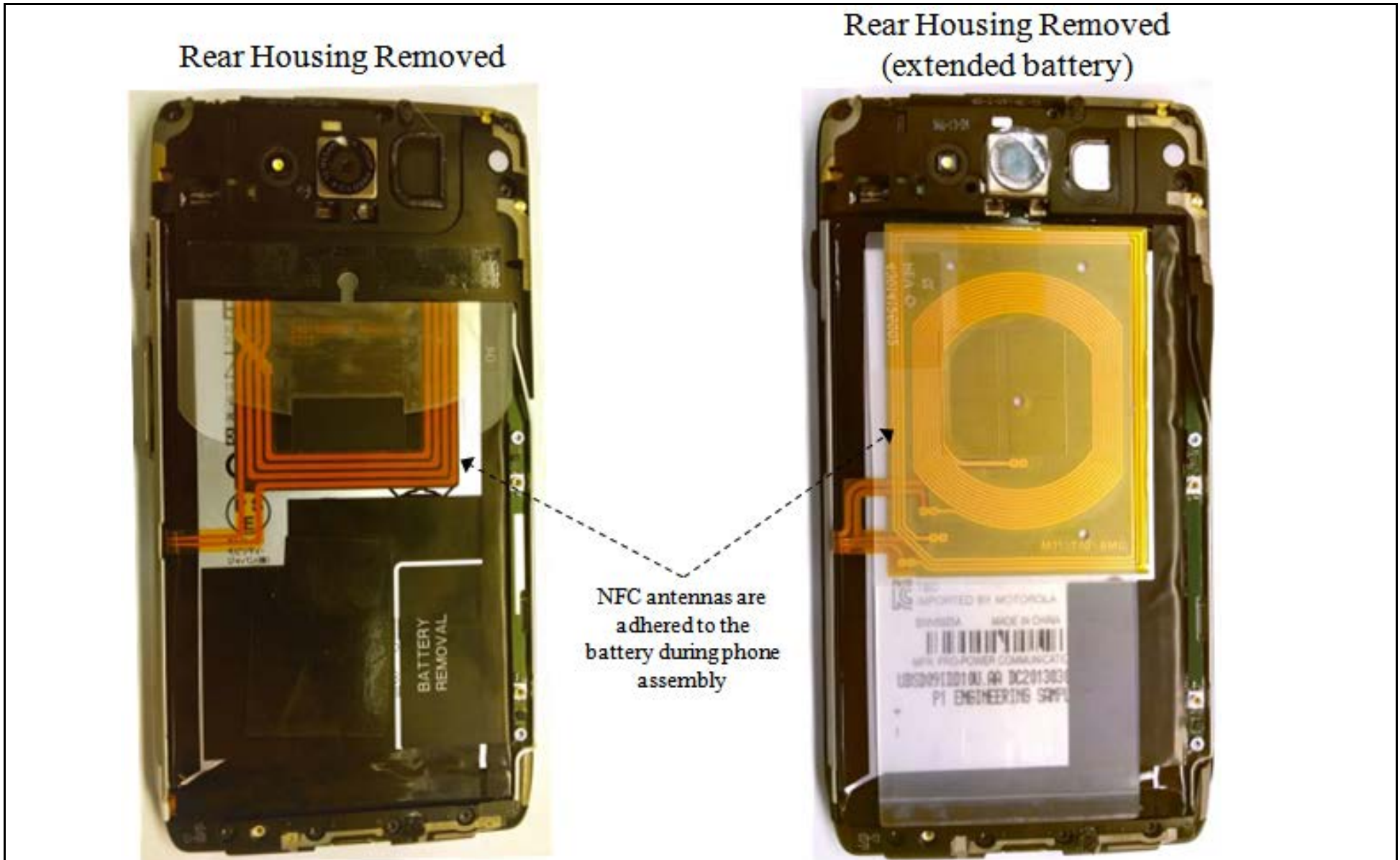
Photograph 9-5: NFC Antenna Locations.
