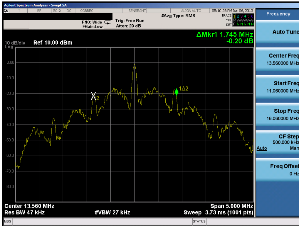
Figure 8-2. 20dB Bandwidth Plot
