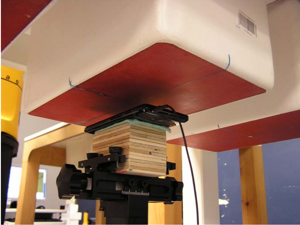
Figure 7: Body Position (25 mm separation, with audio cable shown)
