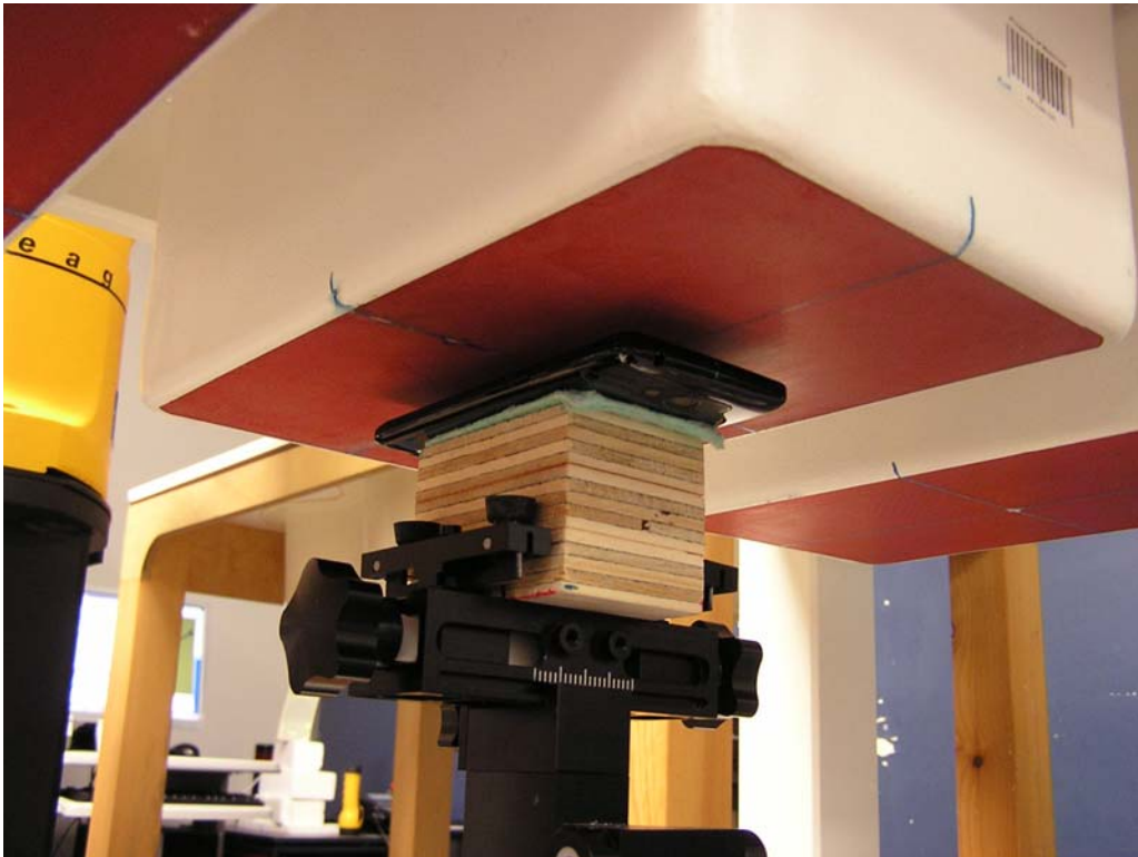
Figure 8: Mobile Hotspot Position, Back of Phone facing Phantom (10 mm separation)
