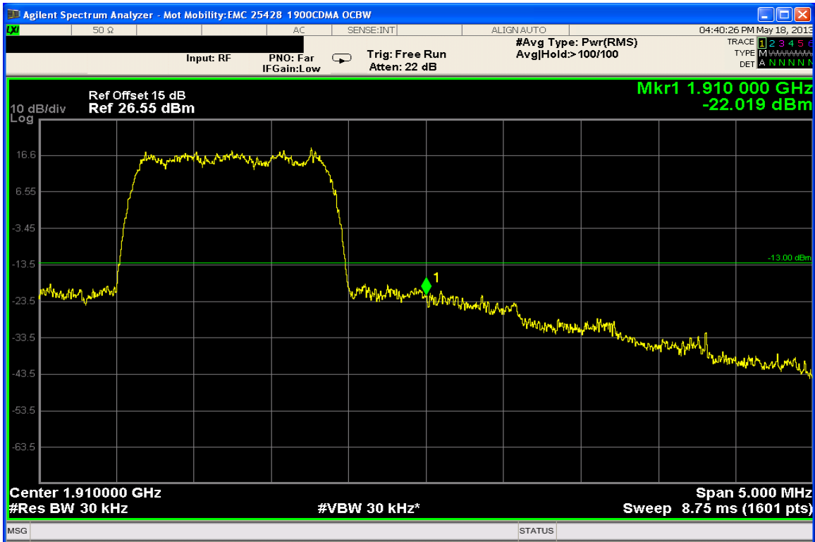
CDMA 1900 – Upper Band Edge – Channel 1175 (1908.75MHz)
