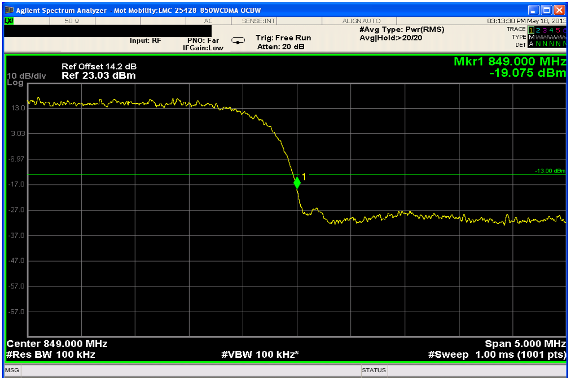
WCDMA 850 – Upper Band Edge – Channel 4233 (846.6 MHz)
