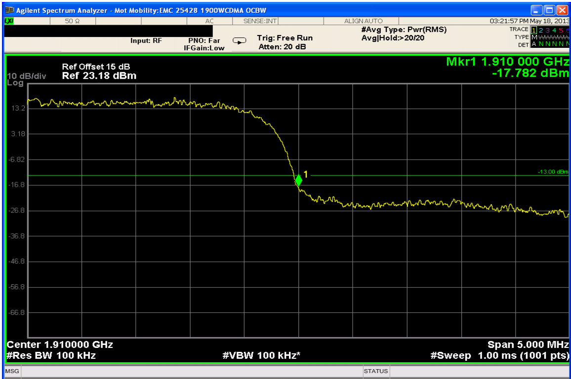
WCDMA 1900 – Upper Band Edge – Channel 9538 (1907.60 MHz)
