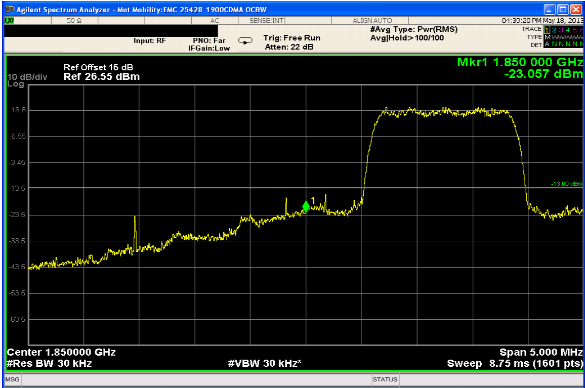
CDMA 1900 – Lower Band Edge – Channel 25 (1851.25MHz)
