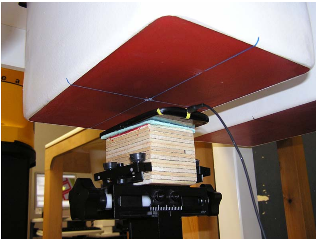
Figure 6: Body Position (25 mm separation, with audio cable shown)
