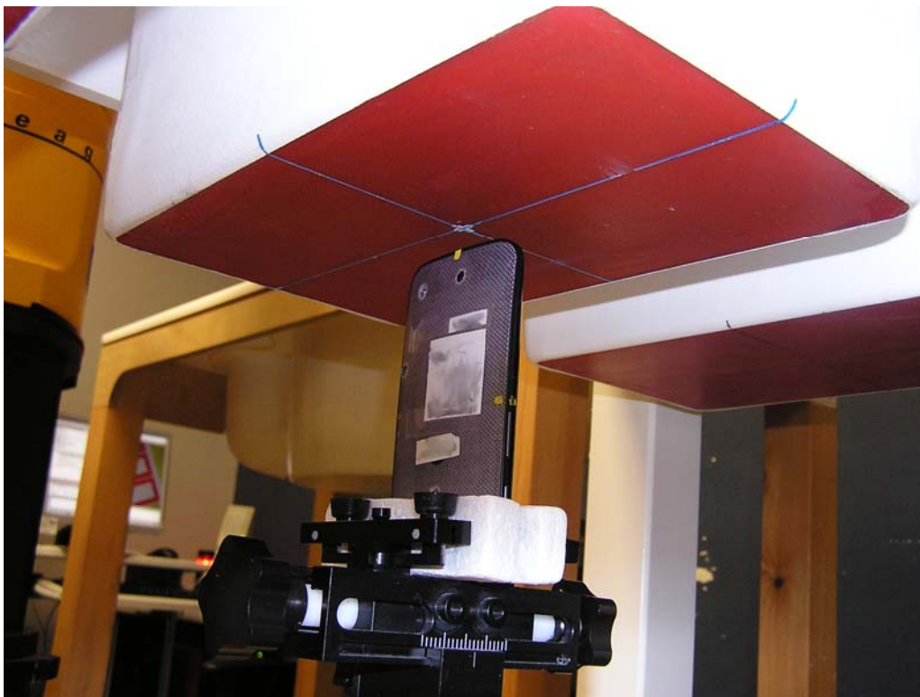
Figure 9: Mobile Hotspot Position, Bottom Edge of Phone facing Phantom (10 mm separation)
