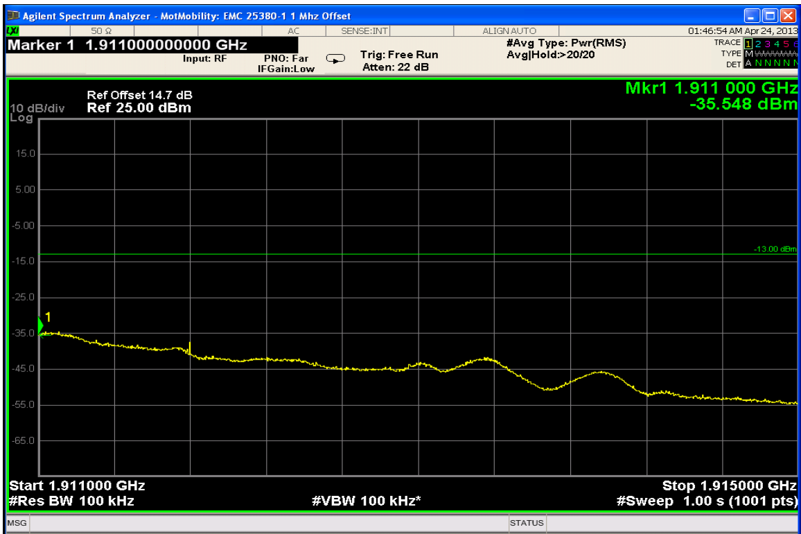
1900 CDMA Conducted Spurious Emissions (Upper adjacent 1 MHz band)
