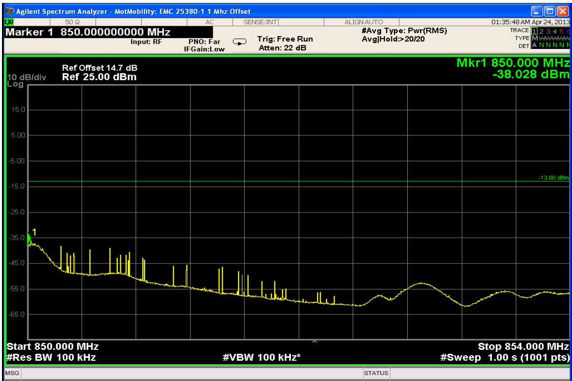
800 CDMA Conducted Spurious Emissions (Upper adjacent 1MHz band)
