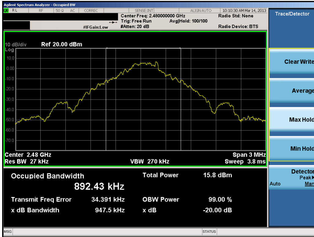
Plot 6-3. 20dB Bandwidth Plot (Bluetooth, 1Mbps – Ch. 78)
