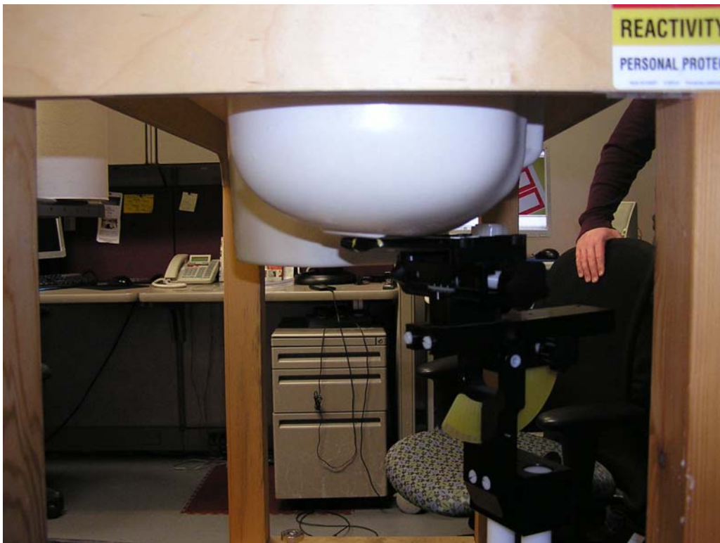
Figure 4: Cheek Position, Top of Head of Phantom
