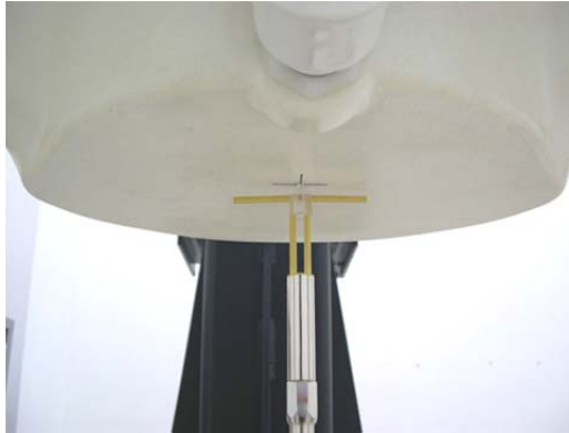
Fig 7.2 Photo of Dipole Setup
