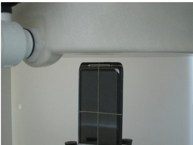
Top Side of the EUT with Phantom 1.0 cm Gap
