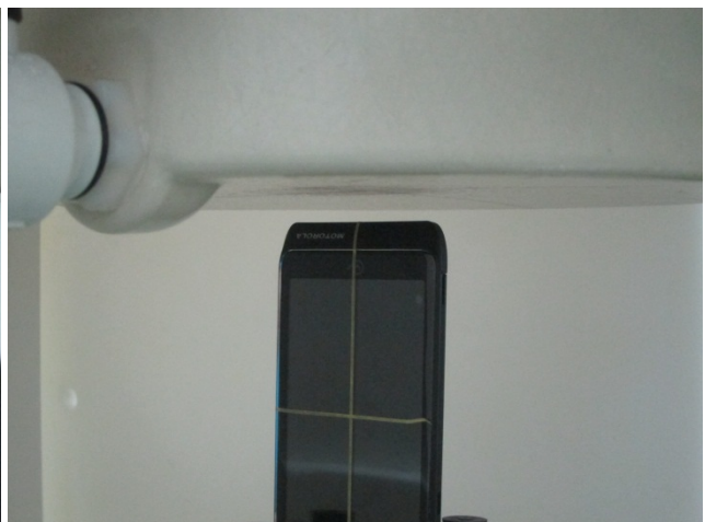
Bottom Side of the EUT with Phantom 1.0 cm Gap
