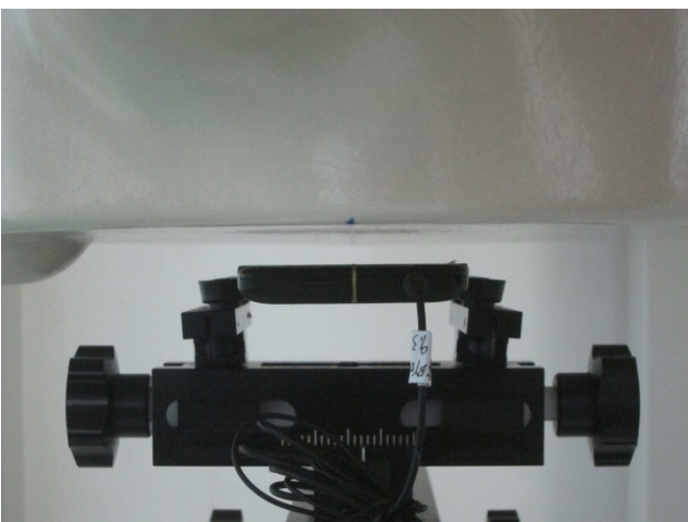
Front of the EUT with Phantom 1.0 cm Gap (with Headset)
