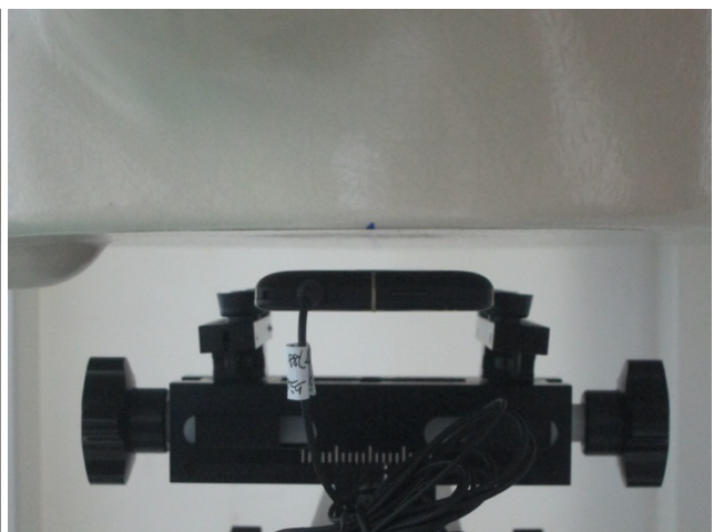
Back of the EUT with Phantom 1.0 cm Gap (with Headset)
