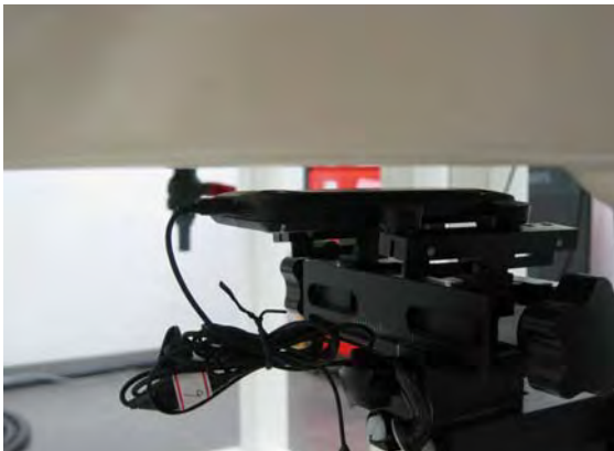
Fig.9 EUT back to flat phantom with headset
