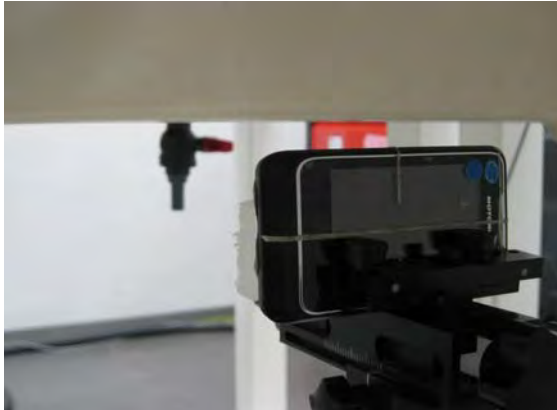
Fig.13 EUT Left to flat phantom
