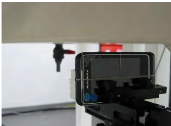
Fig.12 EUT Right to flat phantom
