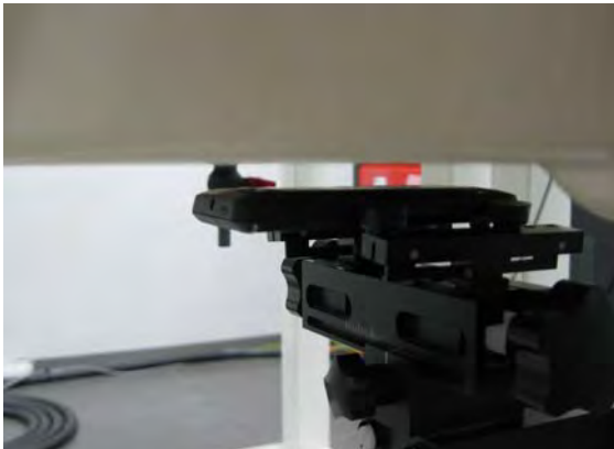
Fig.8 EUT back to flat phantom
