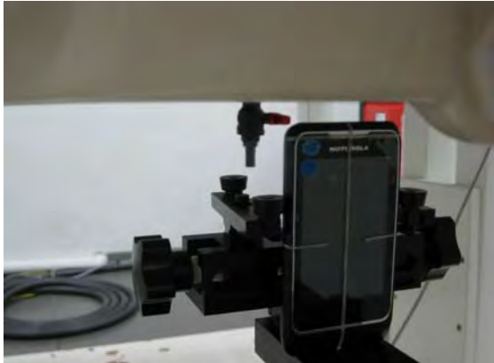
Fig.10 EUT Top to flat phantom
