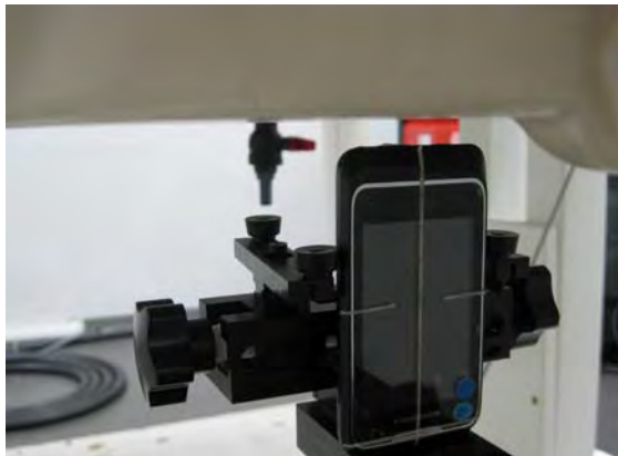
Fig.11 EUT Bottom to flat phantom
