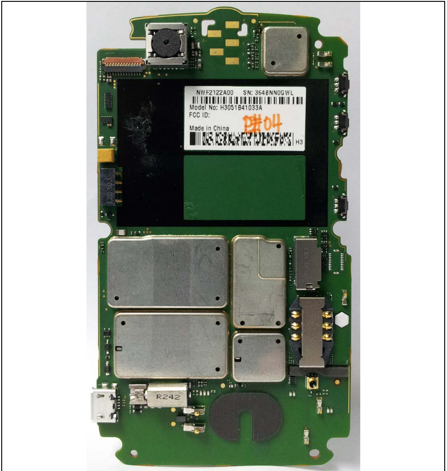
Photograph 9-3: Back side view of the device's PC Board, Shields in place.
