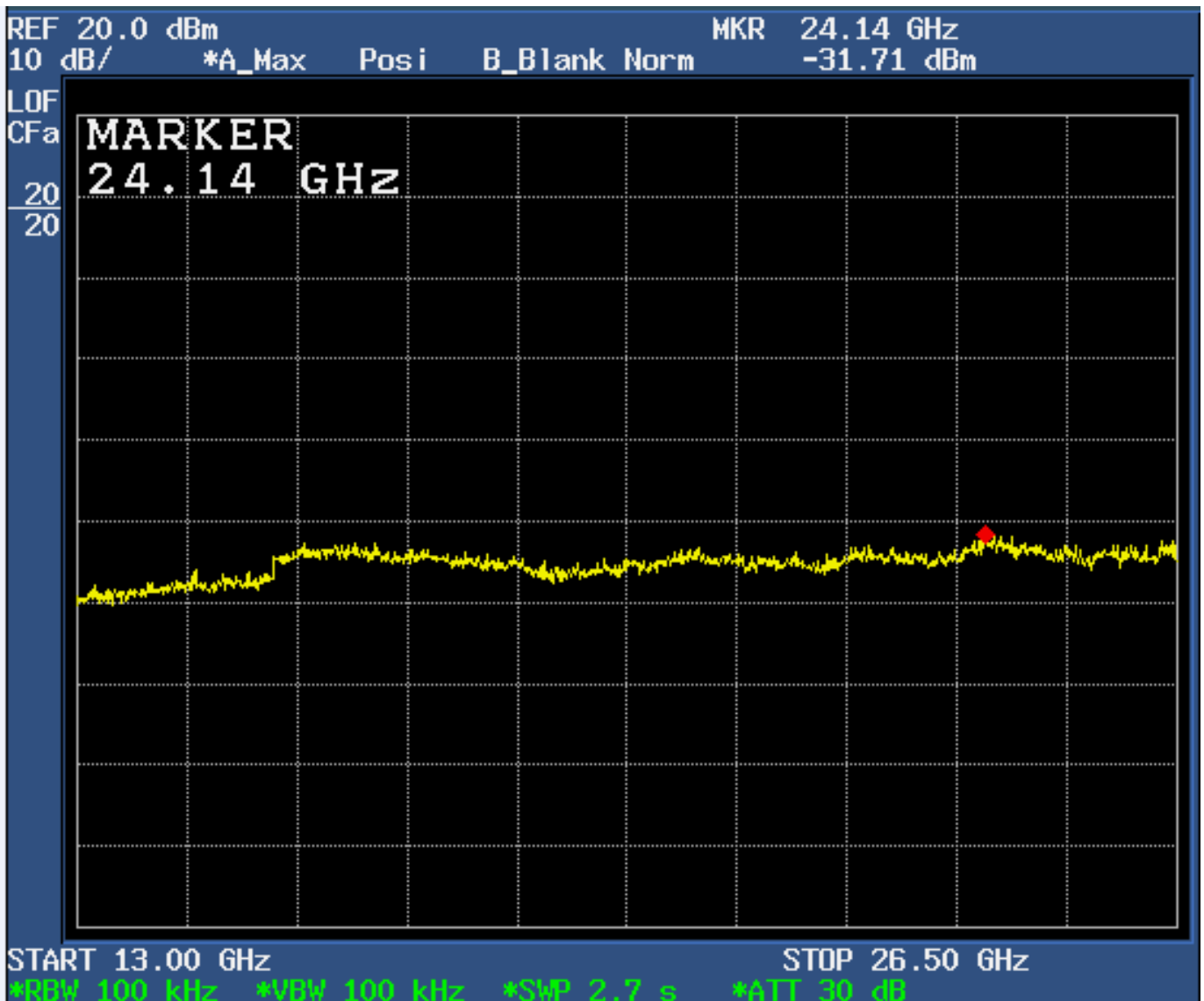
Figure 6d.7-13: Plot of spurious conducted emissions 13.0 GHz – 26.5 GHz (Hopping enabled).
