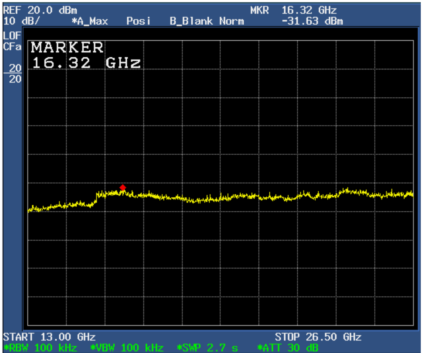
Figure 6d.7-9: Plot of spurious conducted emissions 13 GHz – 26.5 GHz (High channel enabled).
