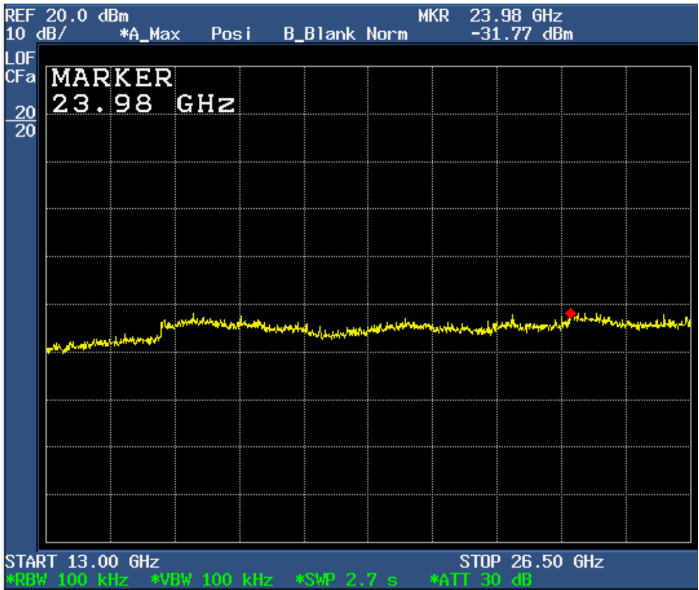
Figure 6d.7-6: Plot of spurious conducted emissions 13 GHz – 26.5 GHz (Mid channel enabled).
