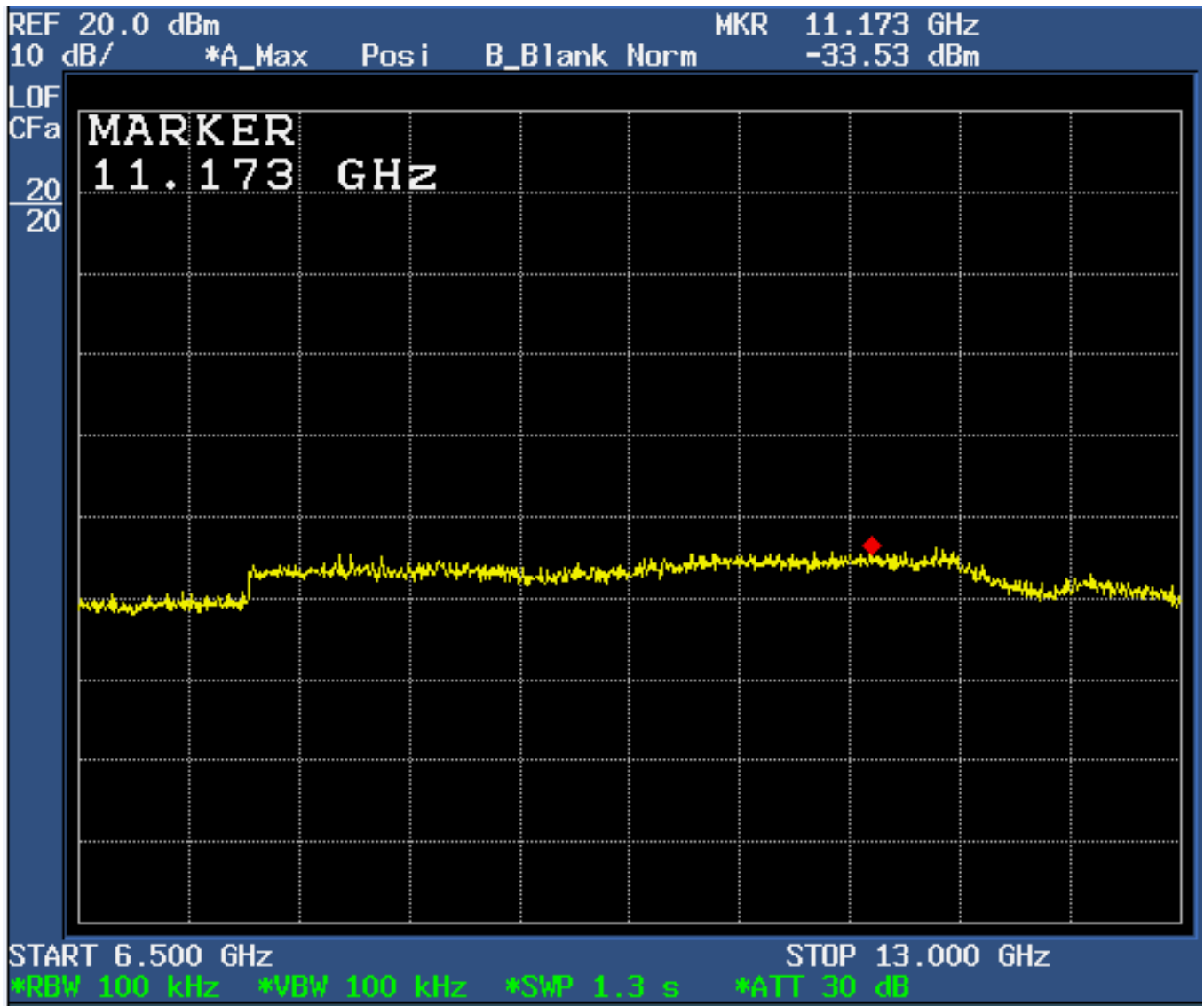
Figure 6d.7-12: Plot of spurious conducted emissions 6.5 GHz – 13.0 GHz (Hopping enabled).
