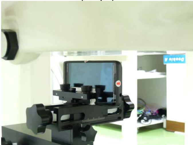
Right Side of DUT with 1 cm Gap (Hotspot)
