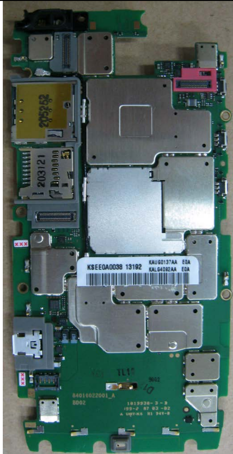
Photograph 9-1: Front side view of the device's PC Board, Shields in place.
