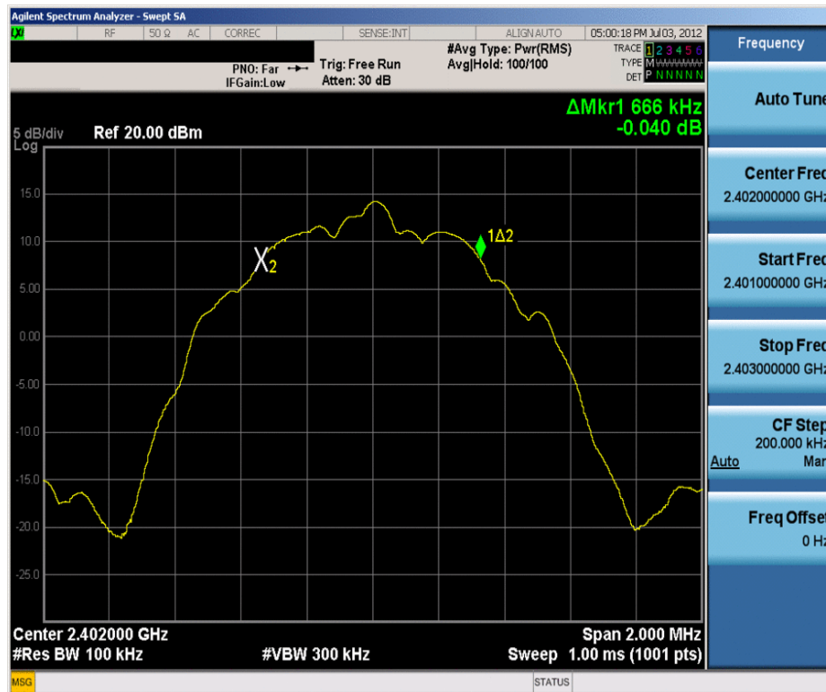
Plot 6-1. 6dB Bandwidth Plot (Bluetooth (LE) – Ch. 0)
