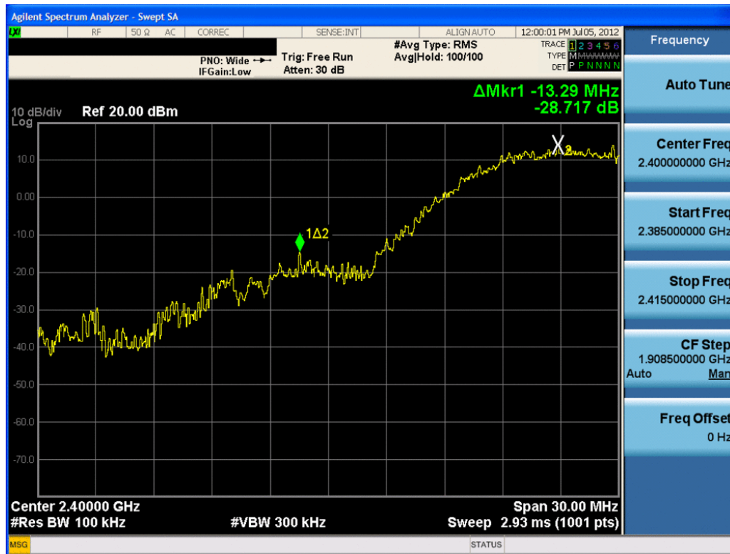
Plot 6-37. Band Edge Plot (802.11b – Ch. 1)
