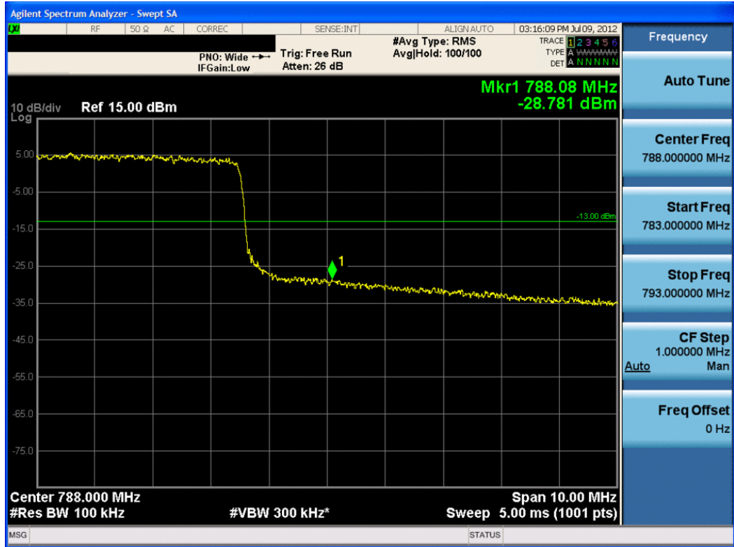
Plot 7-12. Upper Band Edge Plot (16-QAM – RB Size 50)
