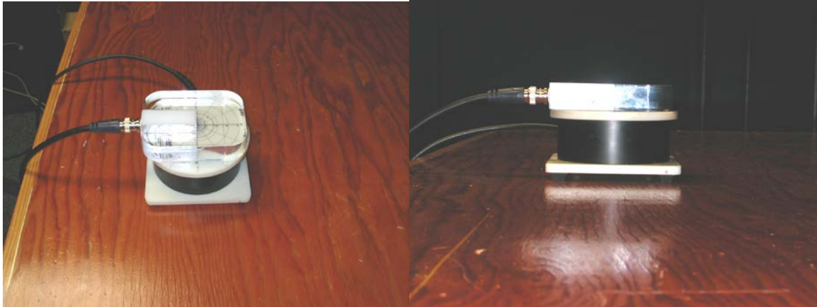
Figure 6-1 – Probe coil being calibrated with TMFS
