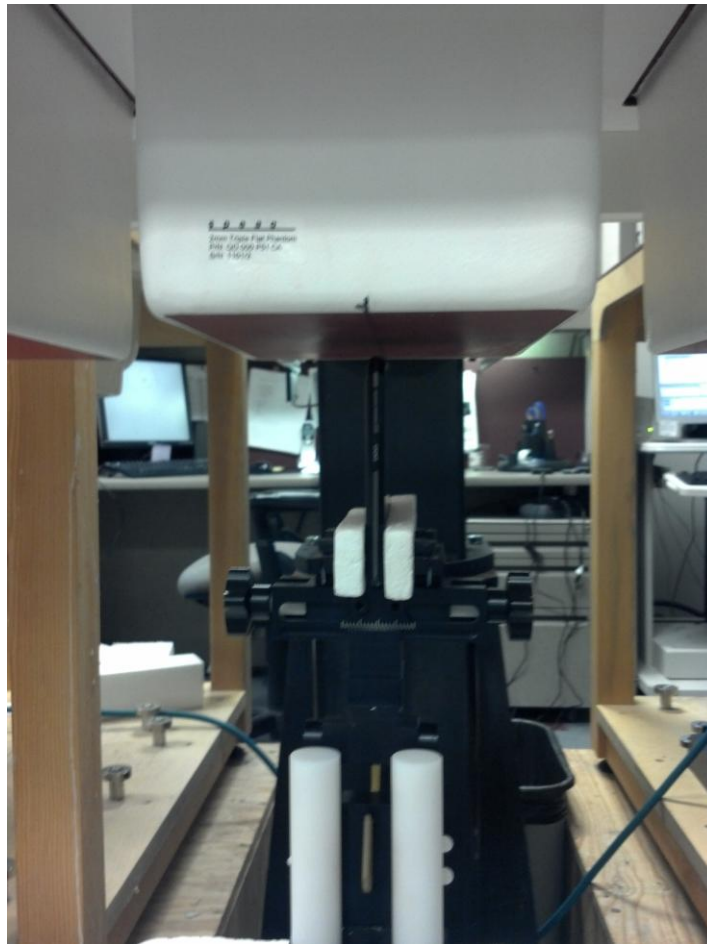
Figure 6: Mobile Hotspot Position, Short Edge of Phone facing Phantom (Top/Bottom)
