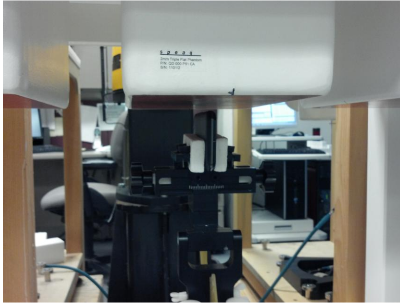
Figure 5: Mobile Hotspot Position, Long Edge of Phone facing Phantom (Left/Right)
