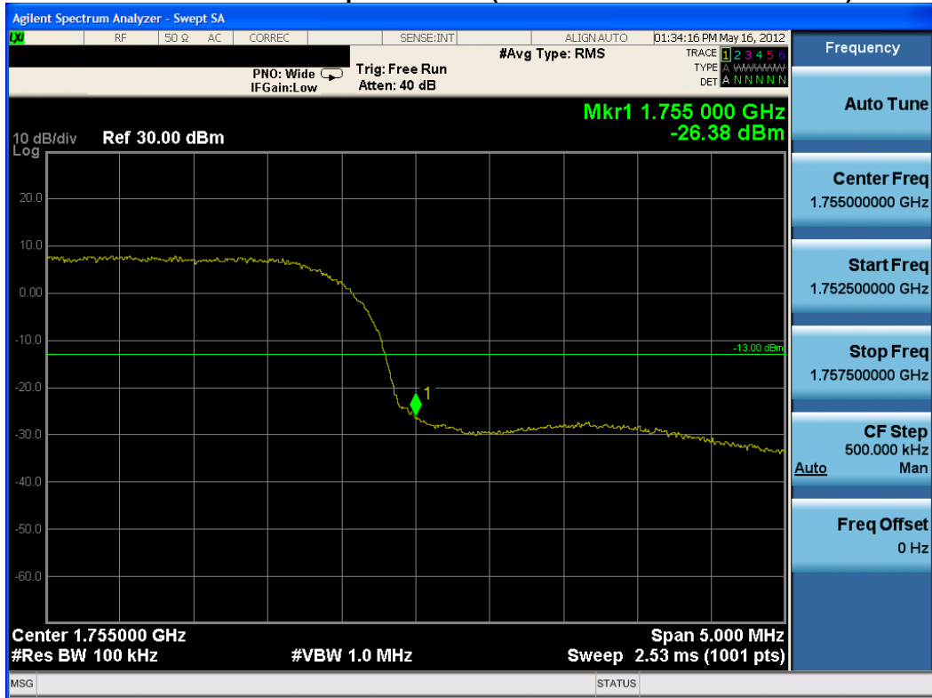
Plot 7-23. Band Edge Plot (AWS WCDMA Mode – Ch. 1862)
