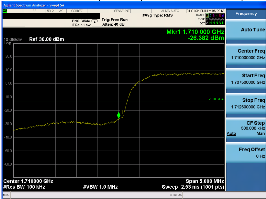
Plot 7-15. Band Edge Plot (AWS WCDMA Mode – Ch. 1312)
