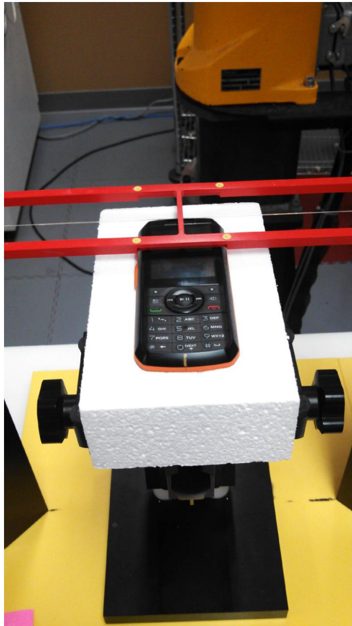
Figure 3. Positioning and Measurement for RF Emissions
