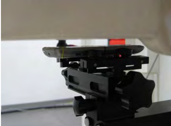
Fig.7 EUT front to flat phantom
