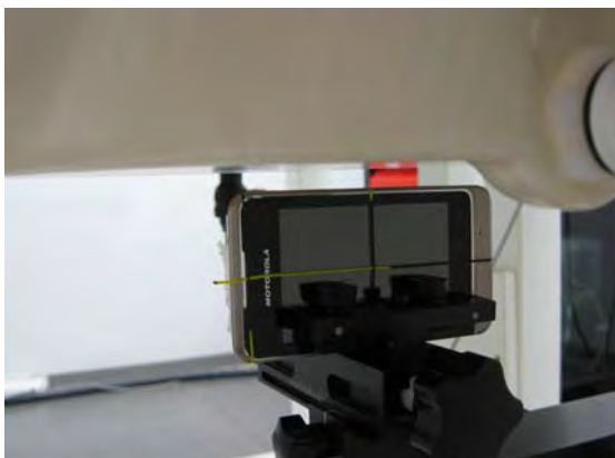
Fig.12 EUT Right to flat phantom
