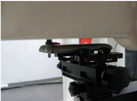
Fig.8 EUT back to flat phantom
