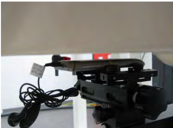
Fig.9 EUT back side with Headset to flat phantom
