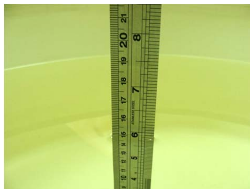
Fig 6.2 Photo of Liquid Height for Body SAR
