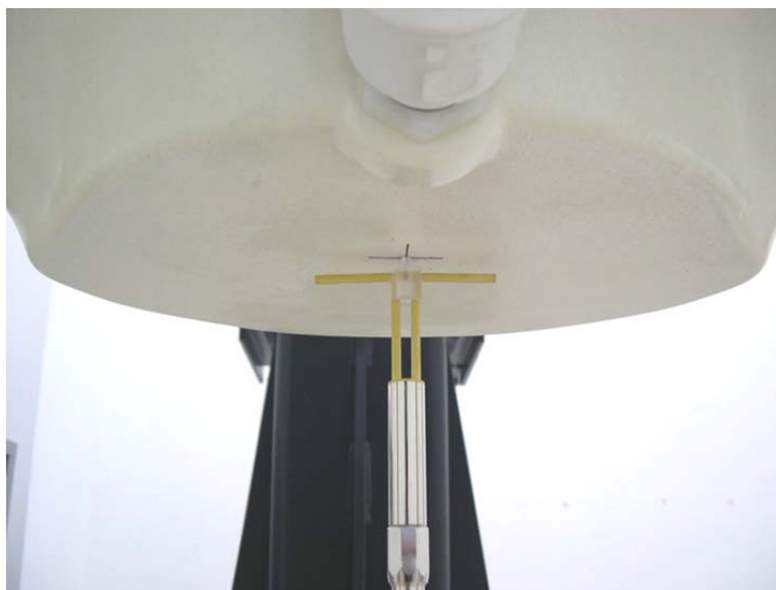
Fig 8.2 Photo of Dipole Setup
