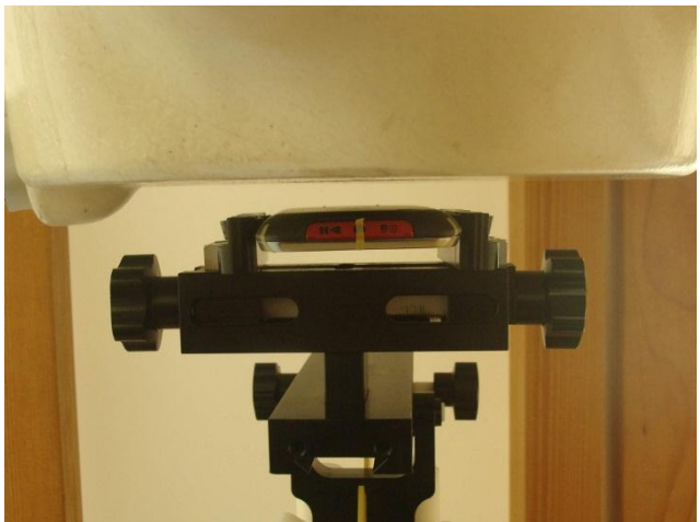
Back of the DUT with Phantom 1 cm Gap (DUT without Earphone)
