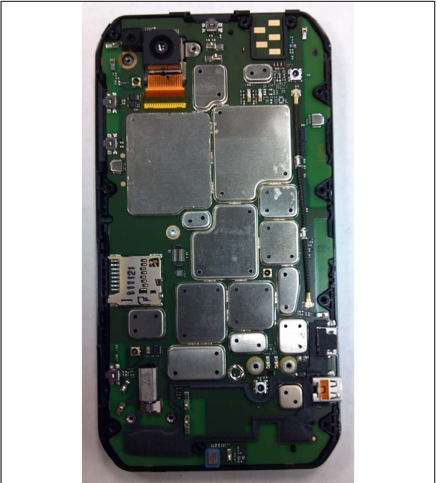
Photograph 9-1: Rear side view of the device's PC Board, Shields in place.
