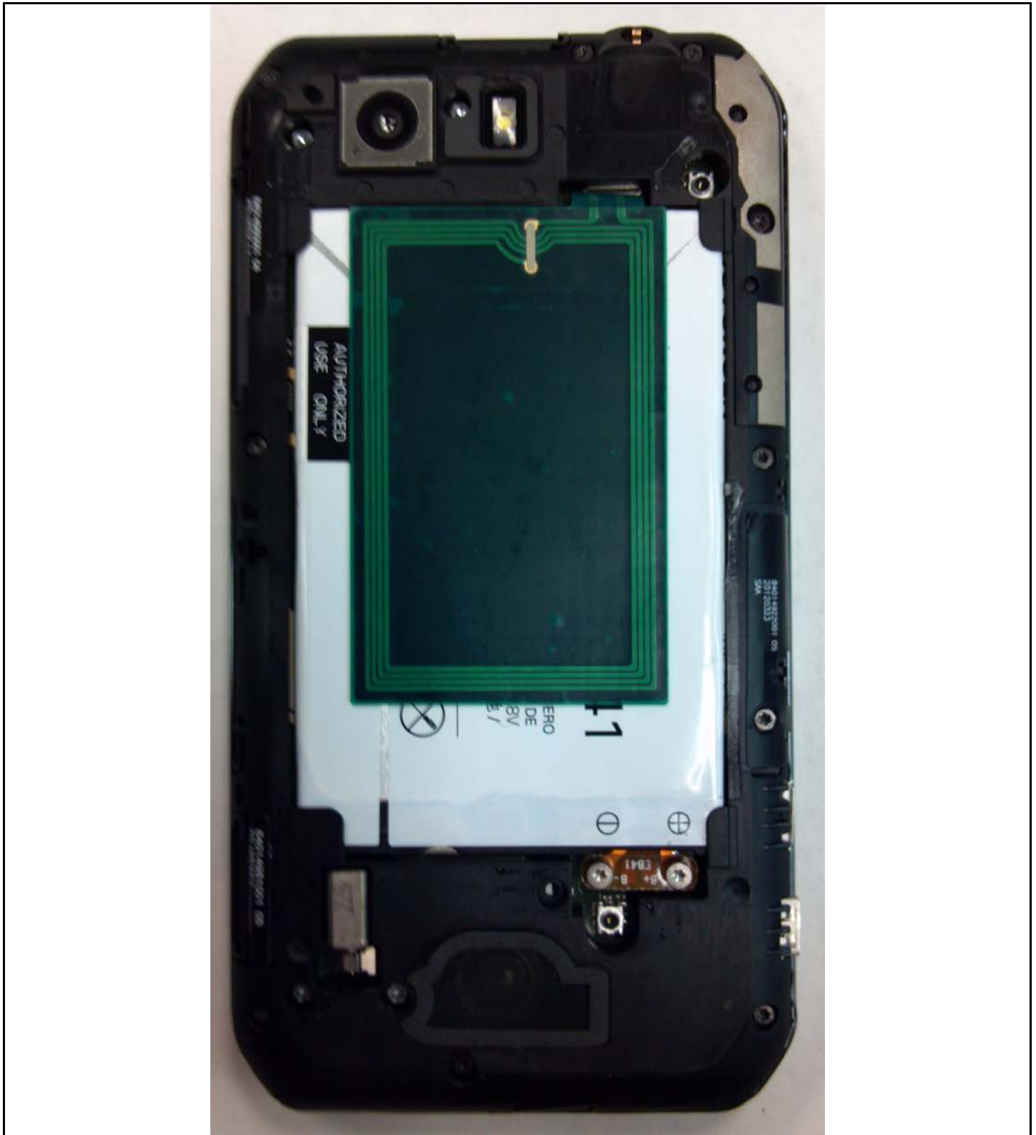
Photograph 9-4: Housing Interior, Showing Integral Battery and NFC Antenna.
