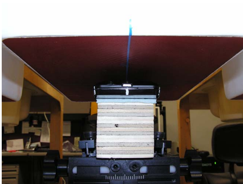
Figure 5: Mobile Hotspot Position, Back of Phone facing Phantom (10 mm separation)
