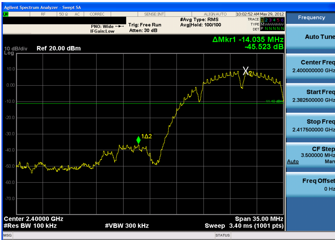
Plot 6-19. Band Edge Plot (802.11b – Ch. 1)
