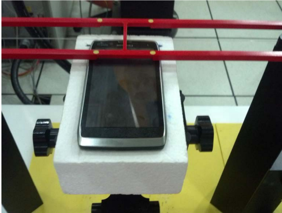
Figure 3. Positioning and Measurement for RF Emissions
