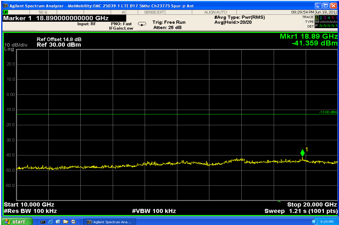
5MHz BW, 16-Qam RB Size = 25 RB Start 0, Low Channel
