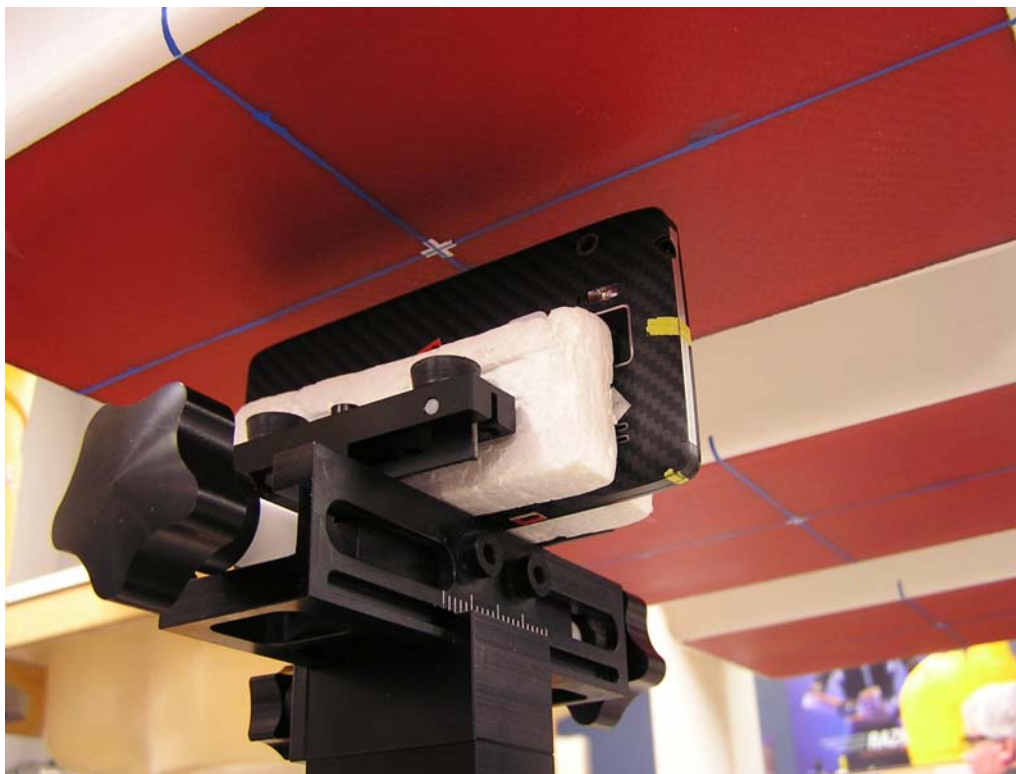
Figure 9: Mobile Hotspot Position, Right Edge of Phone facing Phantom (10 mm separation)
