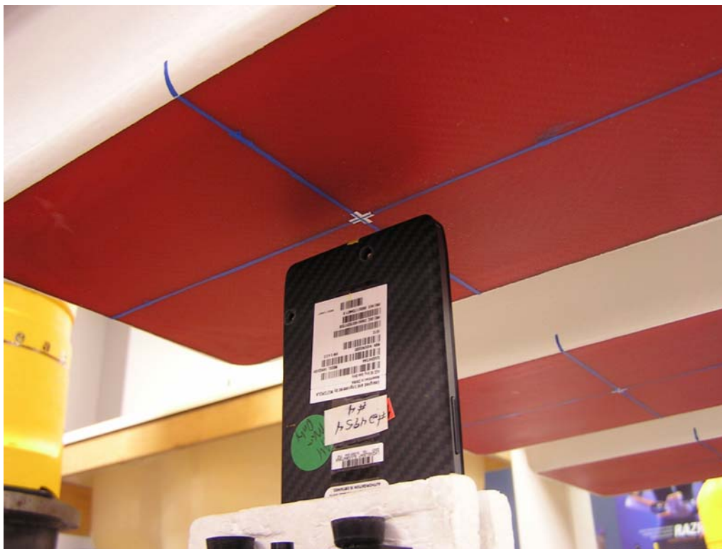
Figure 10: Mobile Hotspot Position, Bottom Edge of Phone facing Phantom (10 mm separation)
