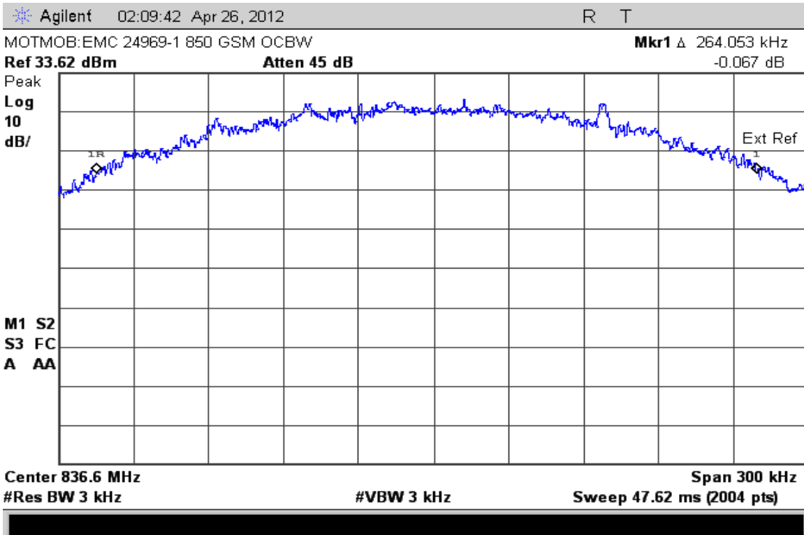
GSM 850 – Channel 190 (836.60 MHz) – Occupied Bandwidth
