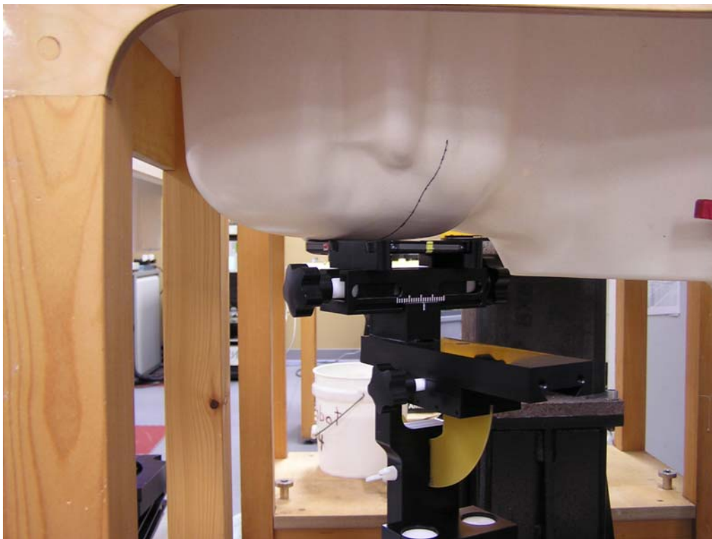
Figure 3: Cheek Position, Front of Head of Phantom
