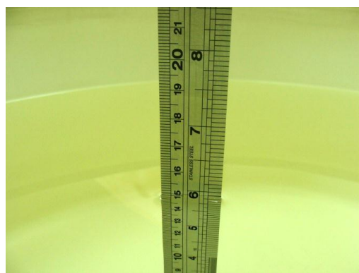
Fig 6.2 Photo of Liquid Height for Body SAR
